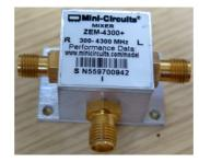
Figure 31.16: Picture of a radiofrequency mixer.
