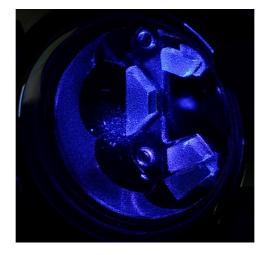
Figure 26.9: Picture of a strontium MOT operated at 461 nm. The atomic cloud, which consists of about  $10^6$  atoms at 5 mK temperature is visible as a diffuse spot located inside a three-mirror ring cavity.
